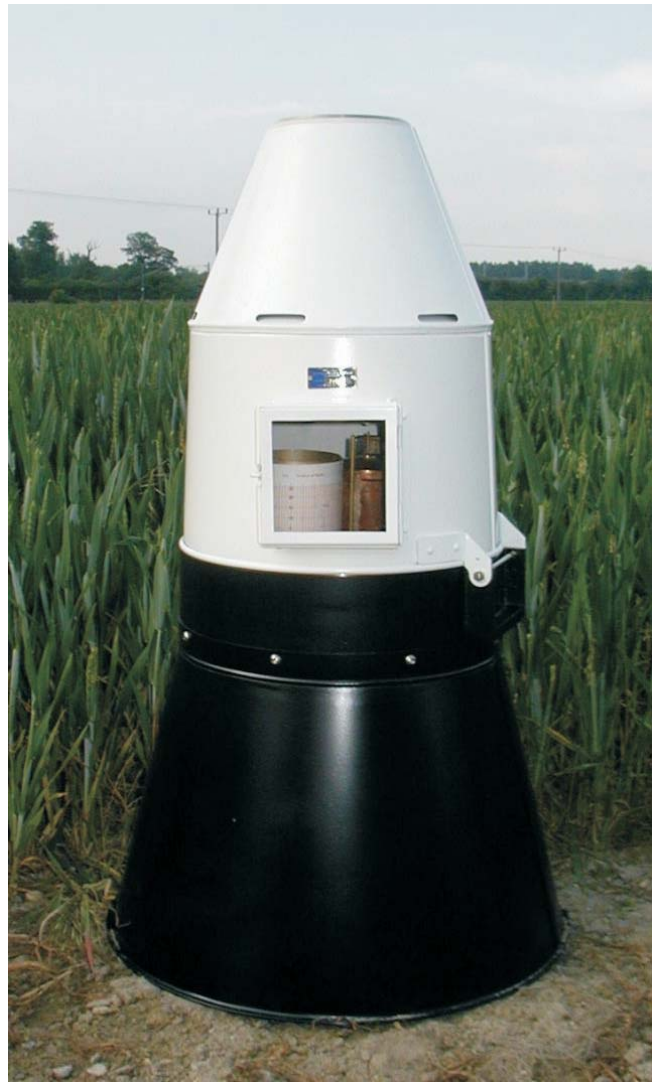
Plate x: Natural siphon rainfall recorder. Source: www.fairmonthweather.com .
