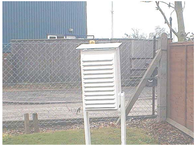
Plate x: Exterior of Stevenson's screen. Source: Http://www.tsrye.fsnet.co.uk/stevensons.htm
