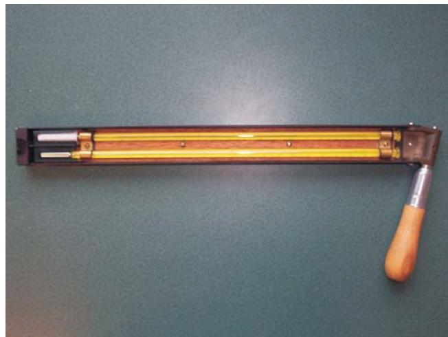
Plate x: Sling psychrometer. Source: http://en.wikipedia.org/wiki/Hygrometer
