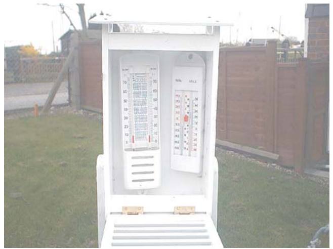
Plate x: Interior of Stevenson's screen. Source: Http://www.tsrye.fsnet.co.uk/stevensons.htm
