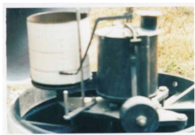
Plate x: Natural siphon rainfall recorder chamber. Source: www.fairmonthweather.com
