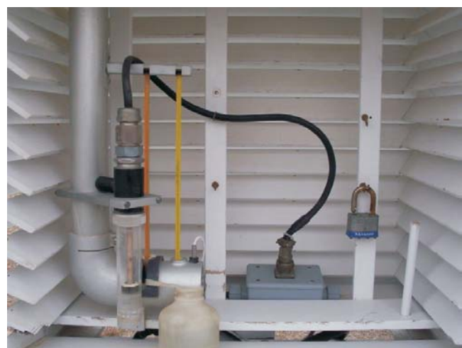
Plate x: The interior of a Stevenson screen showing a motorized psychrometer. Source: http://en.wikipedia.org/wiki/Hygrometer .
